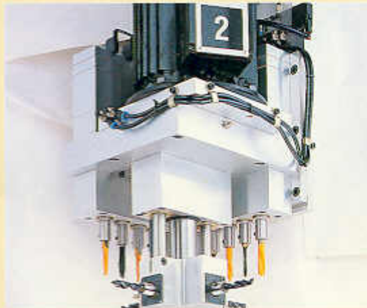
Multifunction drilling unit 11 individually accessible vertical spindles, integrated 4-spindle horizontal drilling head, 4500rpm.
