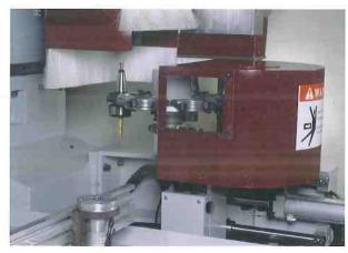
The automatic tool change system provides a 8 positions magazine
