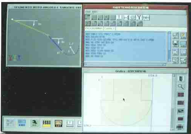
■ Profile Editor for assisted programming and on-line graphics.
