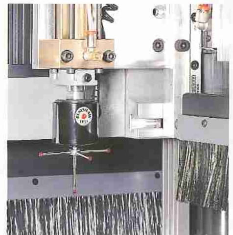
■ Electronic thickness tracer (optional).
