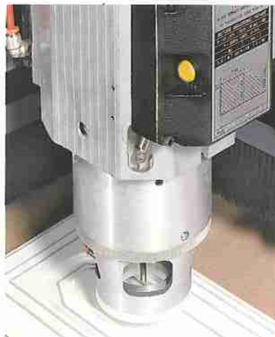
■ Mechanical copying system on Z axis (optional).
