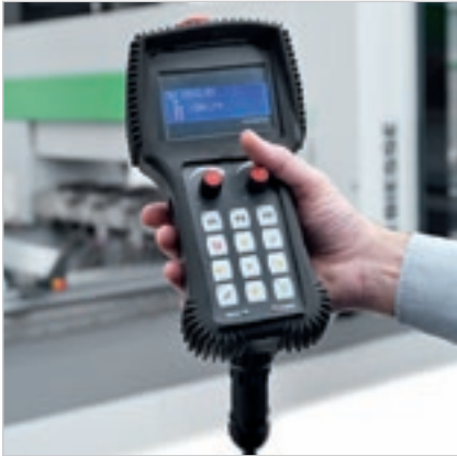
Remote control panel for direct and immediate operator control.
