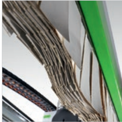
Overlapping lateral curtain guards protect the working unit.
