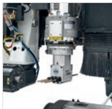
The multi-function unit , which can be continuously positioned over 360° by NC, can house aggregates used to carry out specific machining operations (pocketing for locks, hinge housings, deep horizontal bores, edge trimming, etc.).
