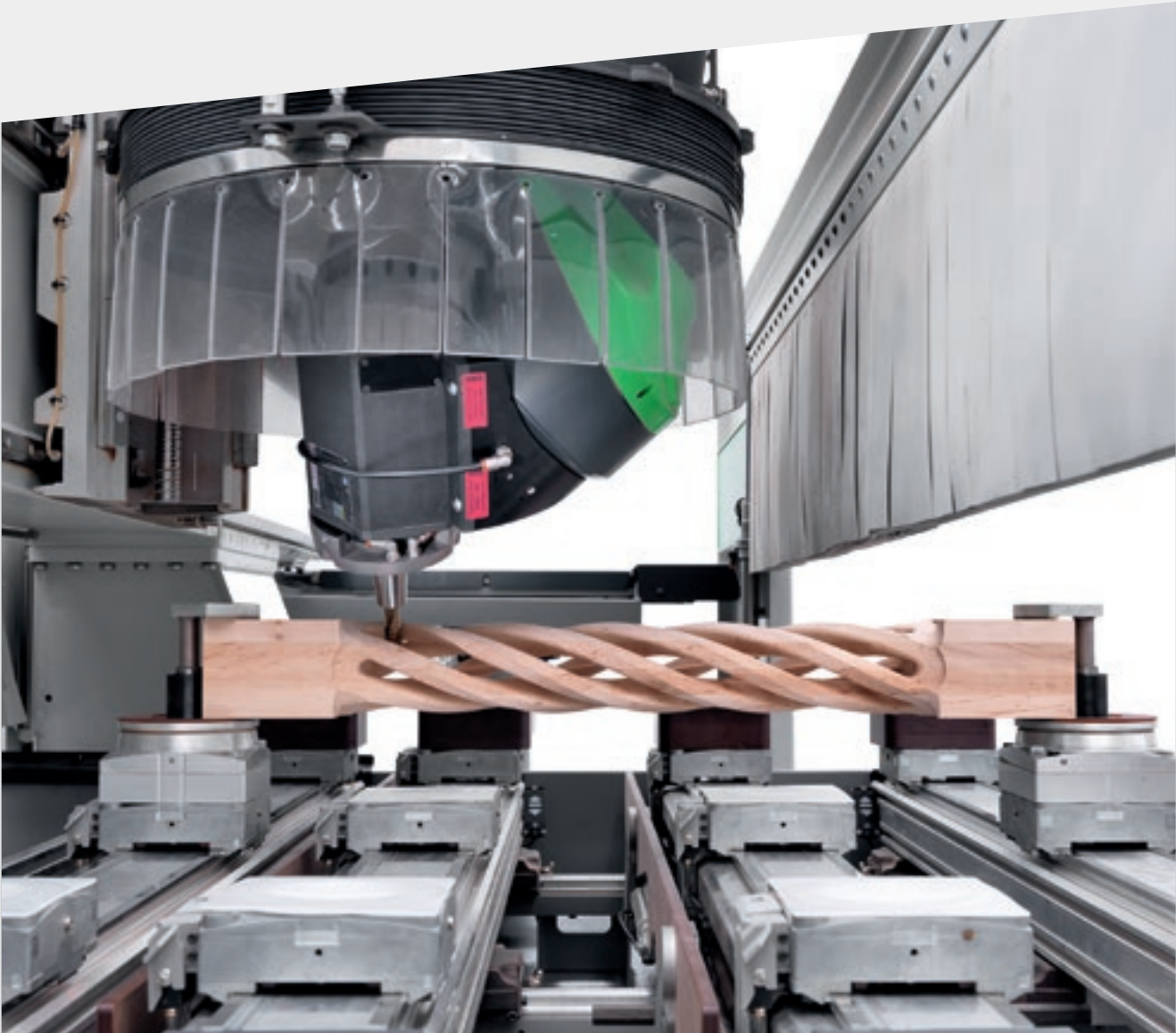
5-axis milling unit with 360mm hood with adjustable height.
