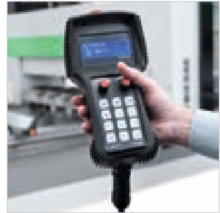
Remote control panel for direct and immediate operator control.
