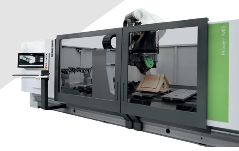
The encasing on this type of machine enables machining operations on delicate, three-dimensional objects, without any risk of damage to the workpiece.
