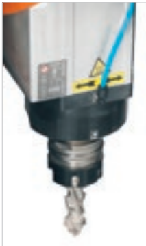
Fixed vertical motor dedicated to additional milling operations (slot, anti-splintering, etc.).
