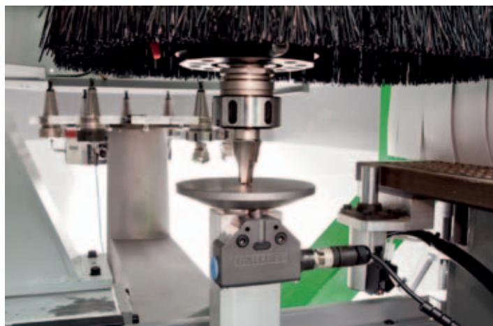
Presetter for the measurement of the tool length.
