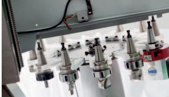
Magazine for tools and aggregates with 12 positions placed on X carriage.
