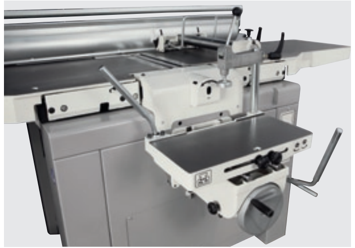
Cast iron mortiser, available on request, with sliding on cylindrical guides and complete with exhaust hood, eccentric pressure beam and 16 mm chuck.
