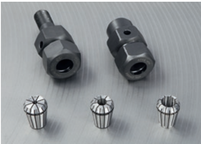
Chuck with clamps 5-10-16 mm, available on request.
