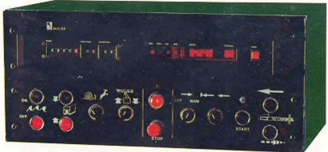
**P1** – Electronic programmer for one size of cut (which can be repeated up to 99 times)
