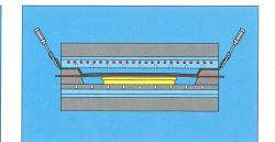
The model for pressing of veneers with membrane. If you want to process veneers only, this model is the most economic one for you. In connection with the heated bottom plate many parts can be pressed both sides simultaneously if the bottom side is not profiled.
