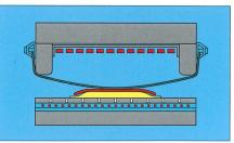
MFP 30/MF was especially designed for veneering. Today veneers can be applied with nearly all membrane presses; but only special machines guarantee most efficient economy at highest quality. Friz membrane presses MFP 30/MF are used today e.g. for the lamination of raised door panels, two- or three dimensionally shaped furniture parts such as table and desk tops, in the production of coffins, and to a great extent in the automotive industry for veneered components like dashboards and consoles.
