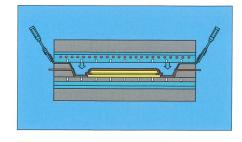
The top-model out of the Optimat program works optional with or without membrane. On this press you can not only produce fronts without membrane, but also economically single doors or samples, or high parts with a specially adapted program, with membrane, or for the lamination with transfer-finish-foils. But naturally you can press veneers as well on this machine.
