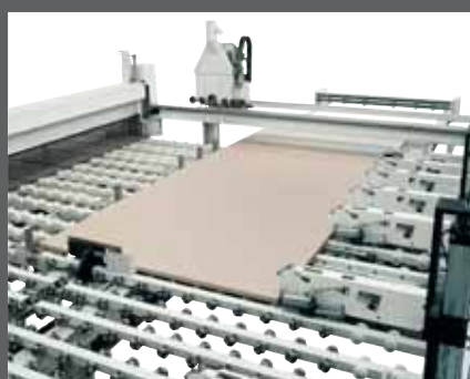
Aligning device with head-cut automatic insertion.
