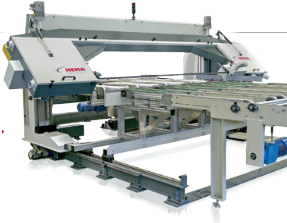
Large width pieces are cut using tilted horizontal bandsaws
