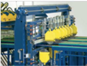
Panel cutting with 14 circular saws
