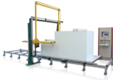
Hot-wire contour cutting of large EPS parts
