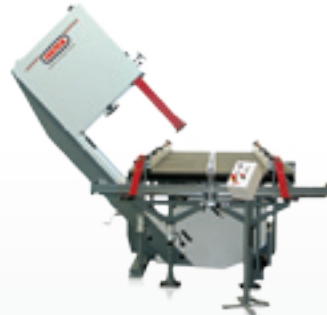
Diagonal cutting of foam glass blocks
