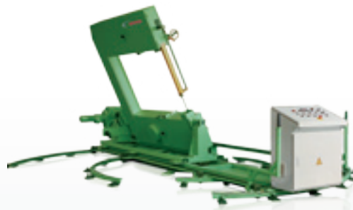
Tilted mitre cutting of large construction elements
