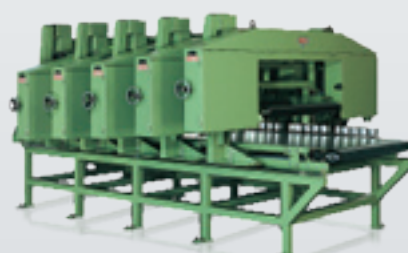
Row of horizontal saws for cutting rock wool panels
