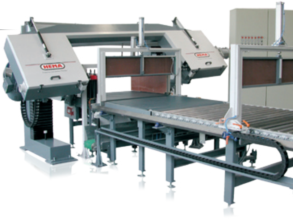
◀ Automatic strip cutting machine for high bulk density products
