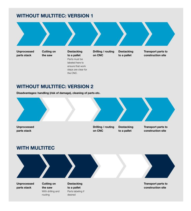
"Drilling on the saw is up to 60% cheaper than conventional drilling. In addition, the SAWTEQ B-300 multiTec is already significantly cheaper to purchase than, for example, the alternative metal processing machines required."
