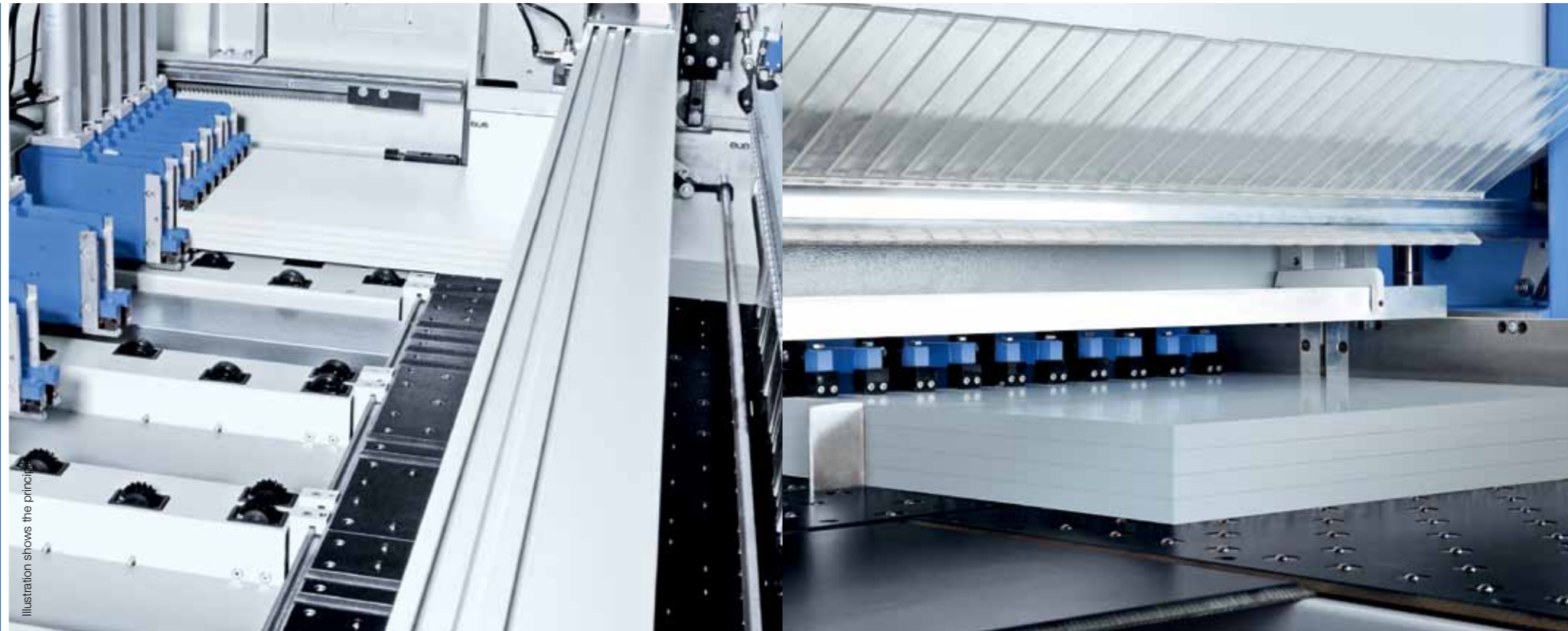
Illustration shows optional equipment: clamps in positions 2 and 4, grooved base plate
