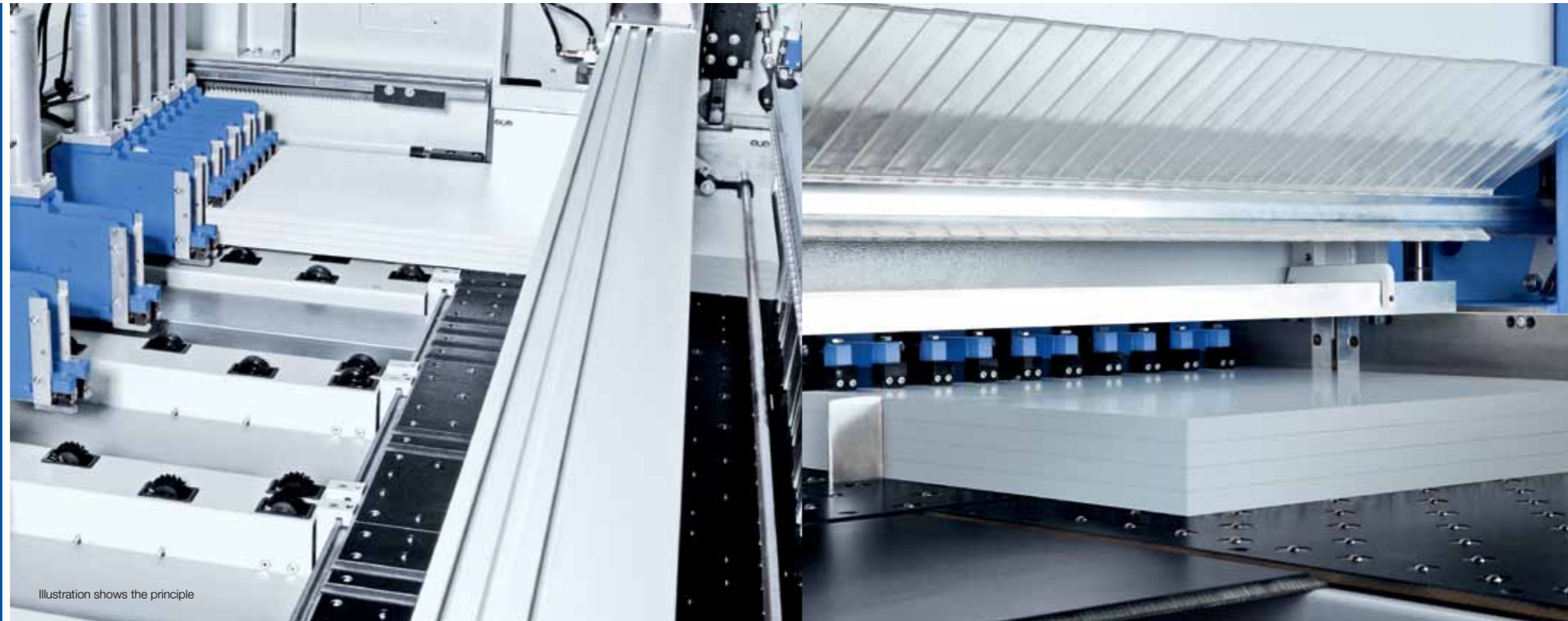
Illustration shows optional equipment: clamps in positions 2 and 4, grooved machine bed plate
