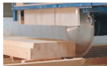
Bevelled saw cuts
