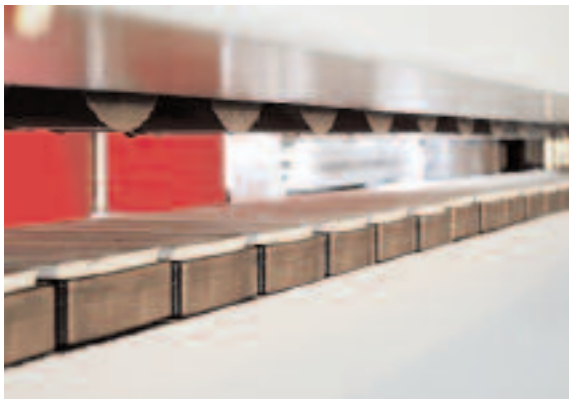
Accuracy right from the start: panel leading and pressure via IMA compound V-belt
