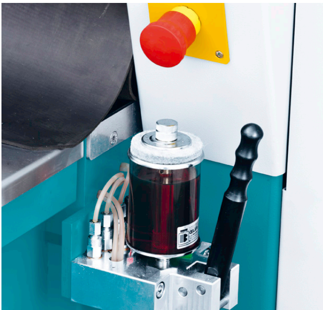
Central lubrication via oil pump
