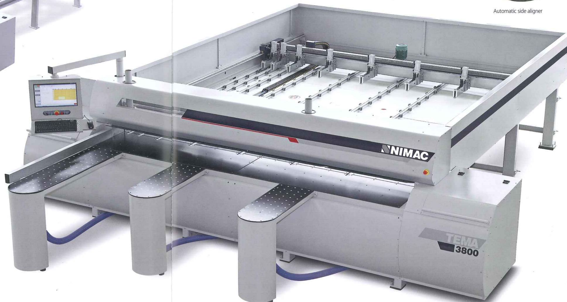
System for grooving cuts in automatic sequence
