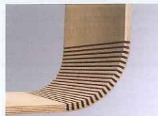
System for grooving cuts in automatic sequence
