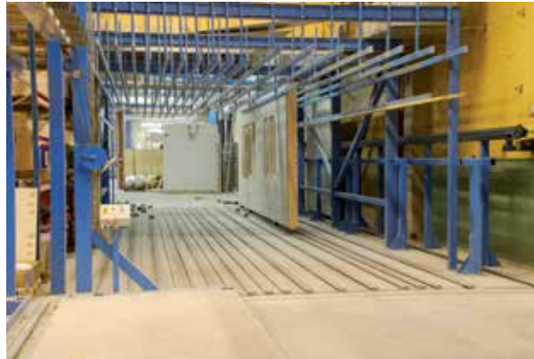
View showing a vertical stock system. Can be fed directly from BS20-system when equipped with option BS2-RVP.
