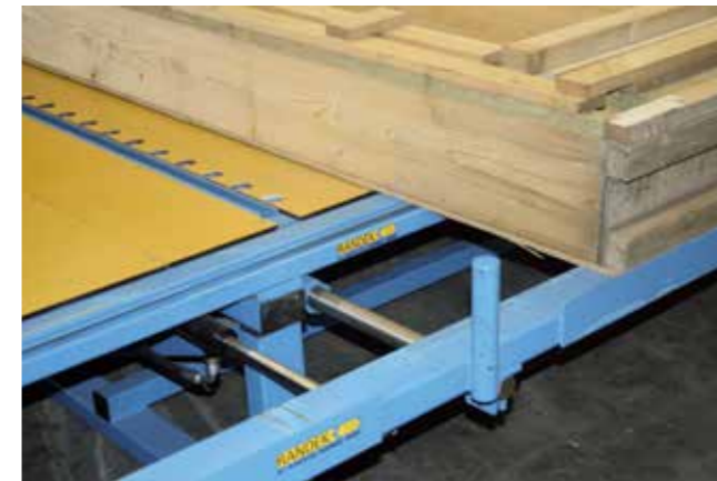
View showing hydraulic width and squaring function (BS2- HW3100HS)
