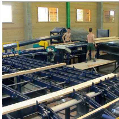
Buffer cross conveyor
