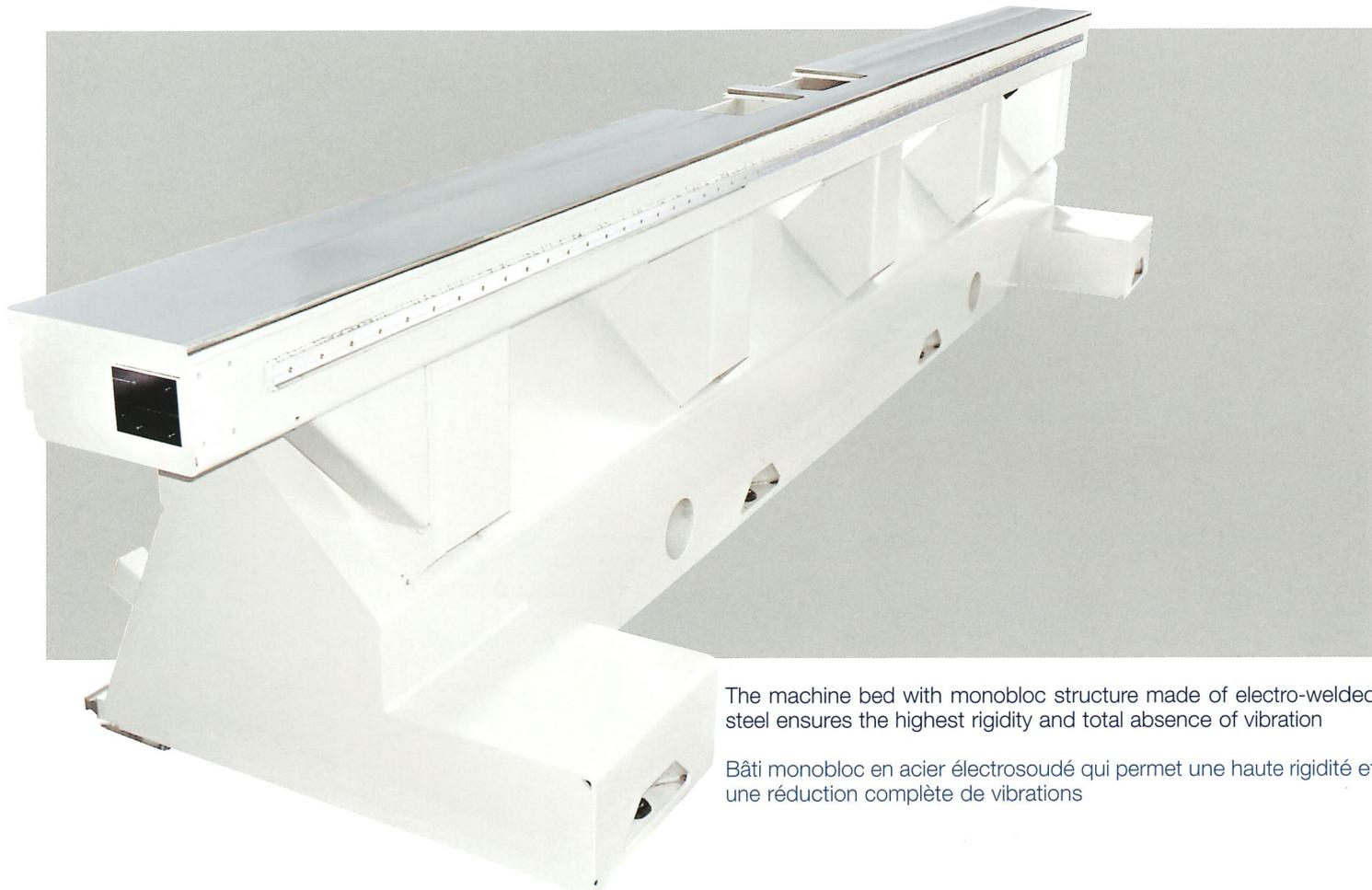
The machine bed with monobloc structure made of electro-welded steel ensures the highest rigidity and total absence of vibration
