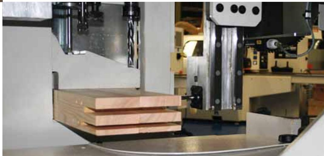
Dogma can be fitted with a drilling-routing unit for all complementary machining when tenoning: the work-piece exits ready to be assembled.
