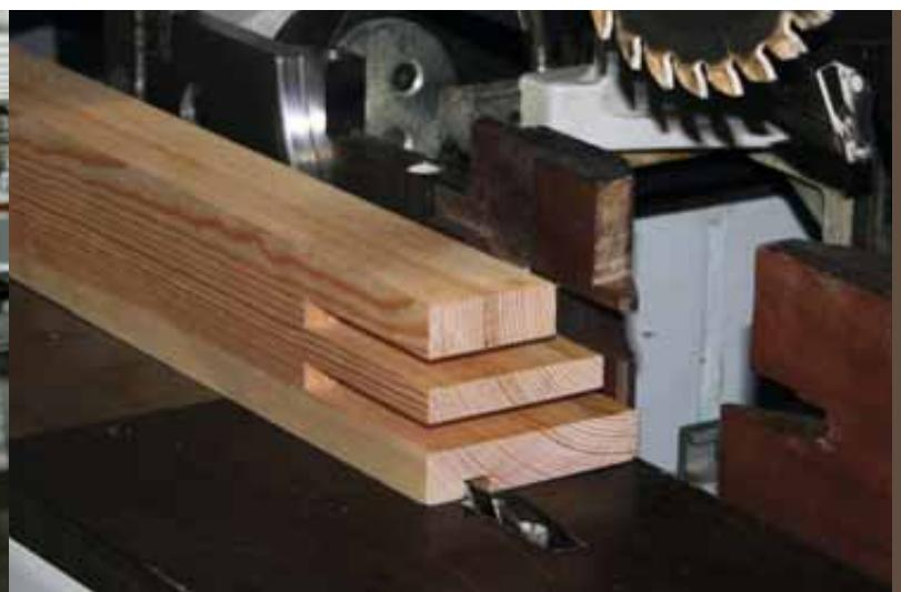
**Bottom horizontal spindle for processing under the work-piece.**
