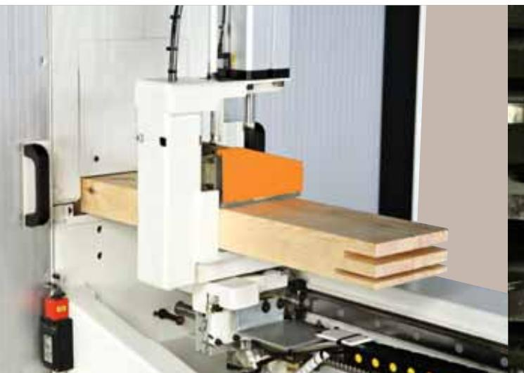
Thanks to the rotary movement of the presser, it is possible to process, in sequence, the two sides of the work piece in a completely automatic way: tenoning has never been so fast!
