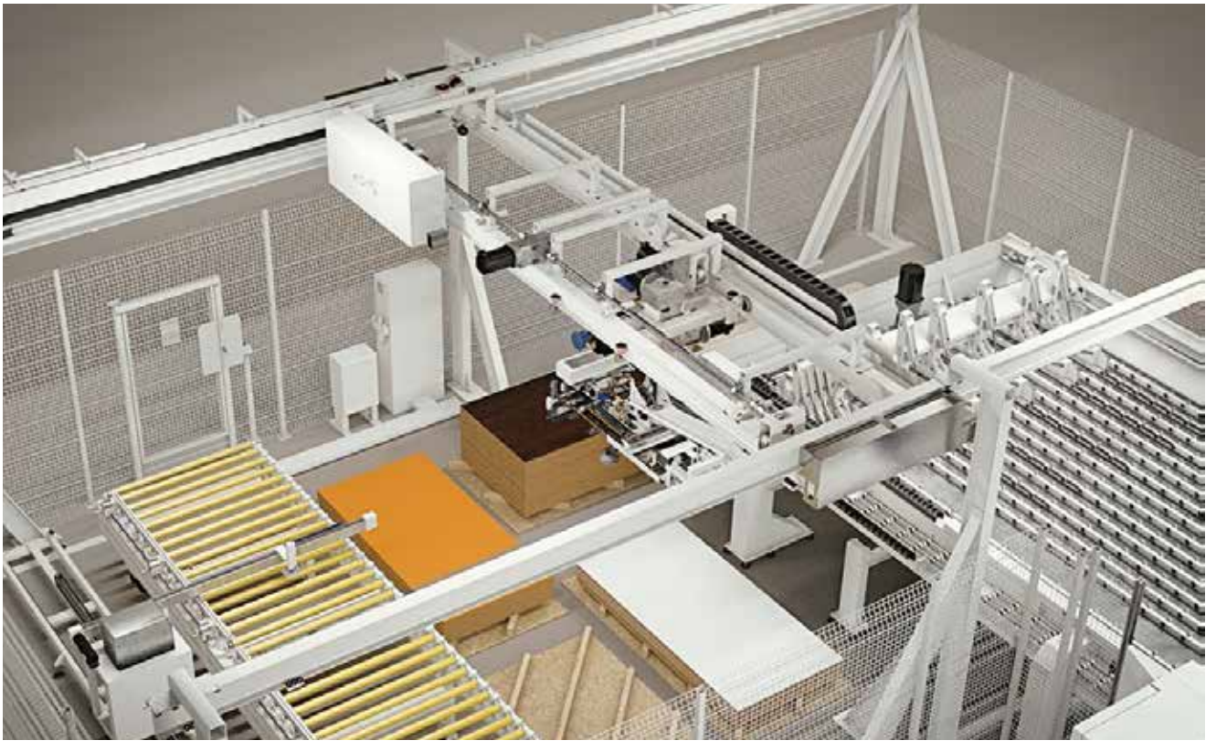
Secure and precise panels transfer. The suction cup arm automatically adapts to the different lengths and widths of the panels to be picked up.
