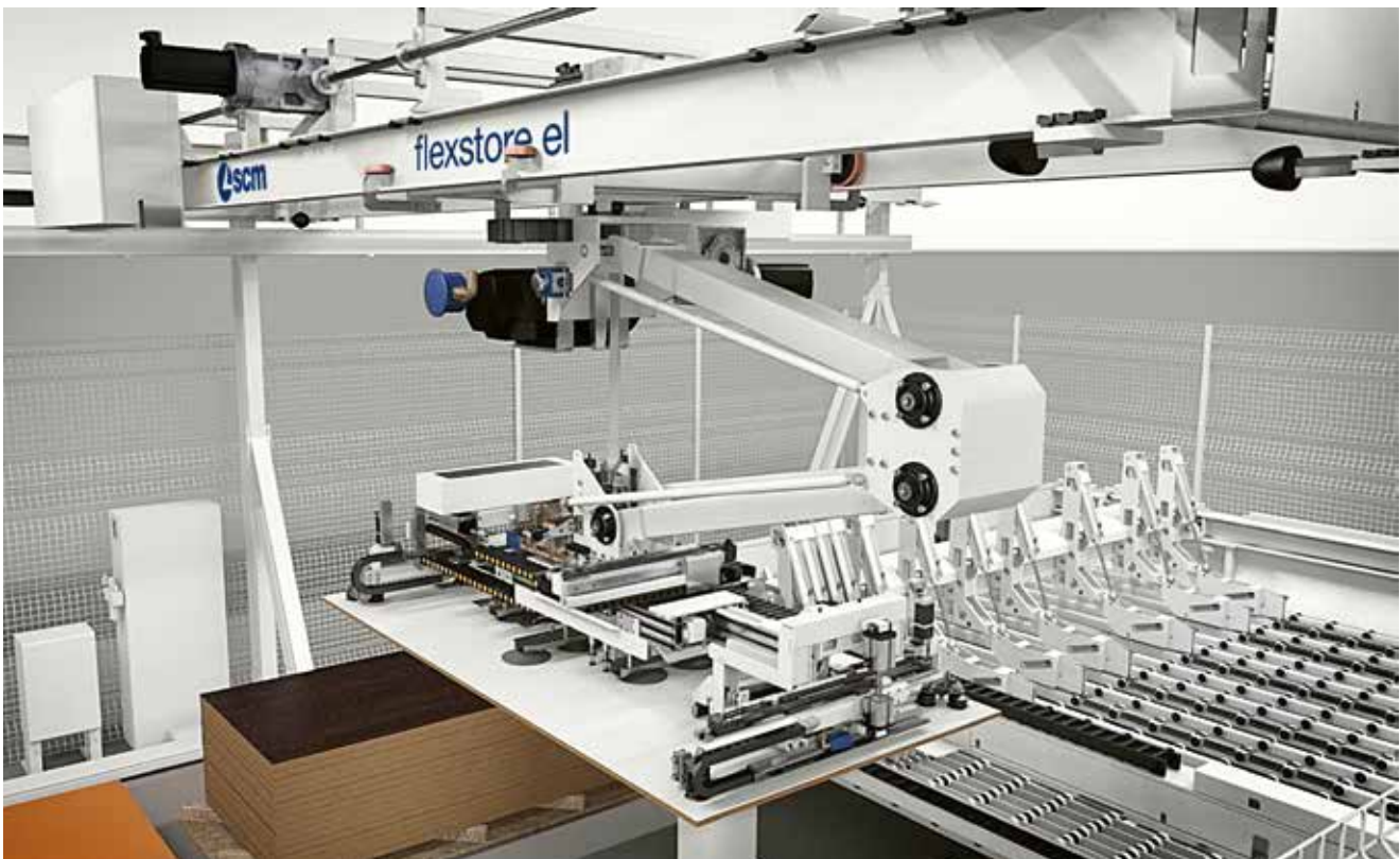
Secure and precise panels transfer. The suction cup arm automatically adapts to the different lengths and widths of the panels to be picked up.
