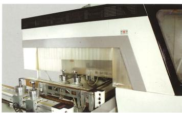
Side protection strips can be excluded by CNC to allow high speed movements.
