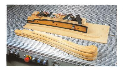
The Multi-function aluminium worktable is machined on the machine itself and guarantees long lasting high precision and flatness thanks to its high rigidity. It is the ideal worktable for machining plastics, resins and light alloys.
