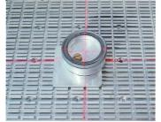
A series of threaded holes (120 mm pitch) provide perfect fixing for all hold-down devices.
