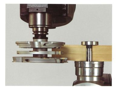
Strong and powerful pneumatic clamps guarantee sturdy component clamping even with high rates of stock removal.
