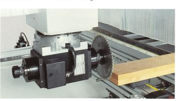
**PBTC**: Auxiliary routing unit with automatic tool changer to ensure the production cycle is faster.
