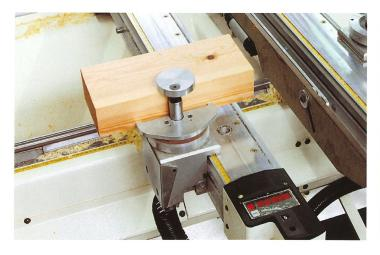
A special pneumatic clamp enables the machining of very short components.
