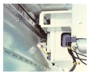
Helical tooth racks for maximum precision on high speed movements.
