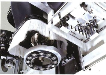
Mechanical presser with ball disc, coaxial to the tool, in order to recover very small components when Nesting machining. The presser strength is regulated pneumatically.
