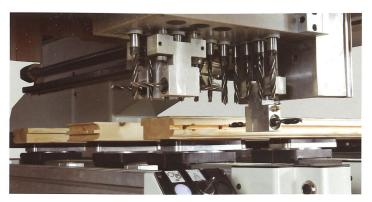
F11, F18, F26: a wide range of drilling units with independent drilling spindles specifically designed for drilling of solid wood.
