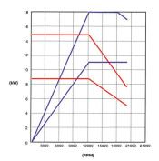
"High power" electro spindles Maximum power up to 20,000 rpm for intensive machining with high rates of stock removal.
