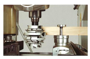
Machining with double profile tool reduces tool changes and increases productivity.
