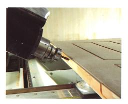
With the Prisma machining head, the same tool can be used horizontally, vertically or in any tilted angle. No need for auxiliary units, the reduction of tool changes and a faster production process.
