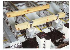
For flexible window production, it is required to have a practical, fast and intuitive system that can quickly fit each window dimension. TVN SET fully meets this requirement: just equip the bars with suction cups or with pneumatic clamps and then modify window dimension data in the parametric program according to size of the window to be machined. The bars automatically position themselves to fit to the new dimensions.
