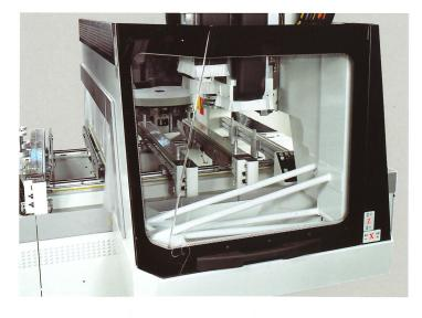
Working unit protection with transparent surfaces to enable the operator to safely view the entire working area.
