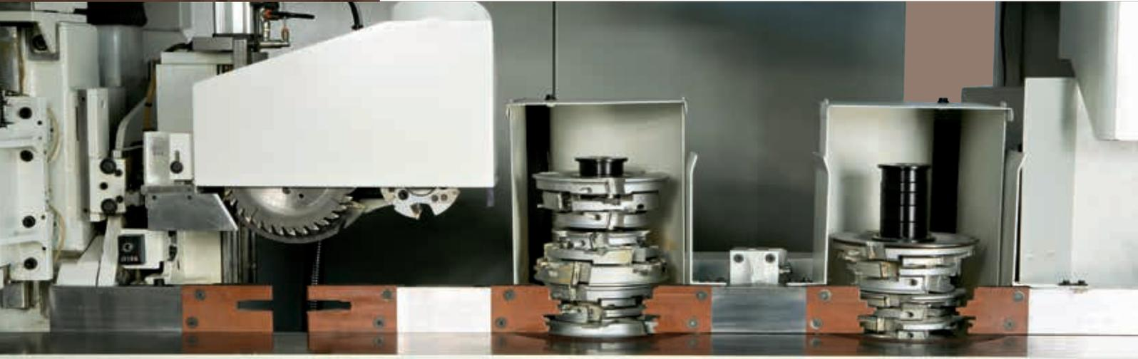
According to profiling requirements two 50x320mm high precision profiling spindles can be fitted on the machine. These groups have 5-position pneumatic horizontal adjustment. They can hold tools with 130/240 mm tool diameter.
