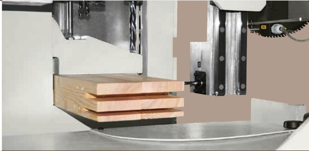
Windor NT1 can be fitted with a drilling-routing unit for all complementary machining when tenoning: the work-piece exits ready to be assembled.
