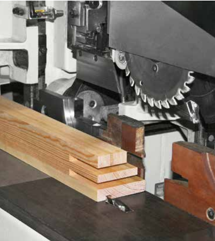
Horizontal spindle for the machining of the bottom side of the work-piece.
