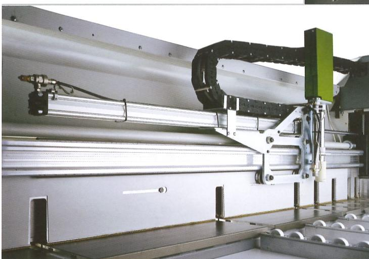
Side alignment is effected by means of a rubberised roller that keeps the material against the square fence, thus guaranteeing the perfect squaring of the pieces being sized at all times.
