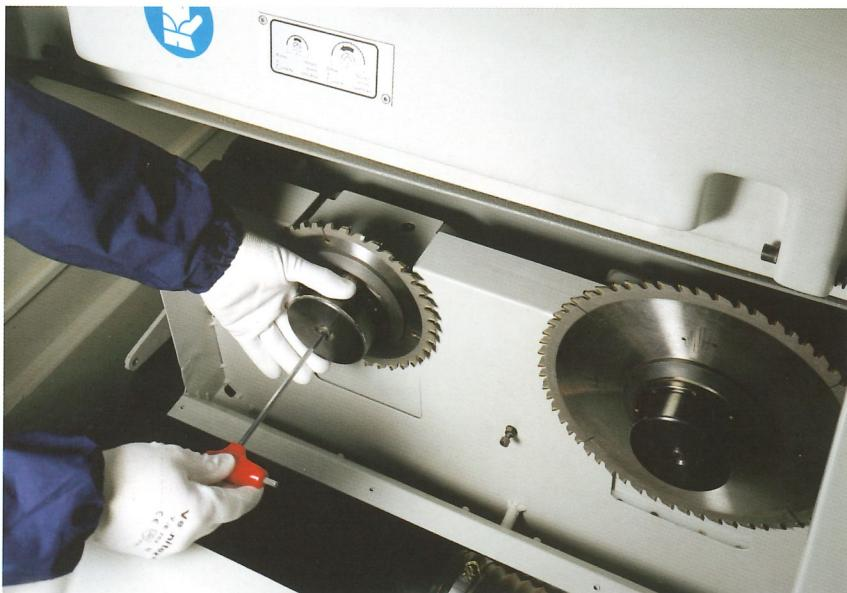
The saw blade change zone is located at the side of the square fence and can be accessed from the front. Tool replacement is carried out using just one wrench and is simple, safe and fast.
