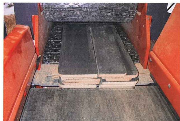
Chain link infeed for timber waste and chipboard stacks
