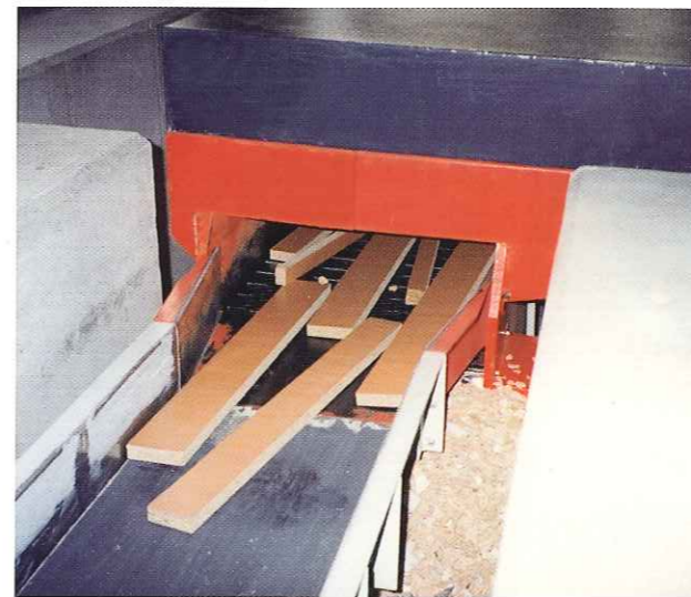
LEOPARD in a pit connected directly to a panel dividing saw
