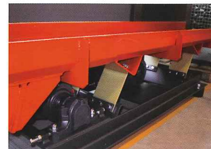
Vibrating chute, electrical drive
