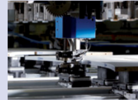
Perfect edge finish due to traced combination flush trimming / scraping unit – efficient processing without tool change.
