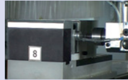
Aluminium thread tapping
