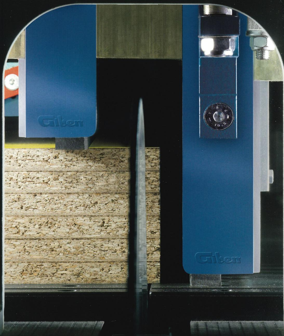
*The double pressure beam represents the solution for effective dust emission control, by lowering on the base during trim cuts and creating a TUNNEL for dust extraction. The perfect and even contact of the pressure beam on the entire surface of the stack and the pressure beam with no cut-outs ensure a higher cutting quality.*
