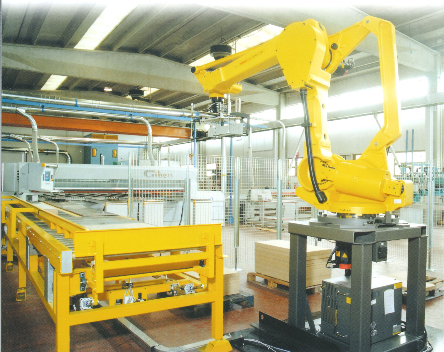
The picture shows a solution of sorting and unloading of the parts.
