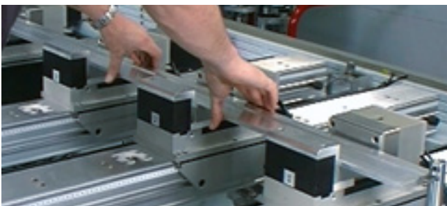
Special clamping elements for aluminium processing
