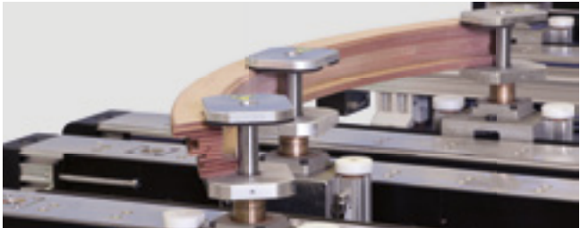
Sash bar insertion aid: Special inserts for sash bar clamping simultaneously act as insertion aids.
