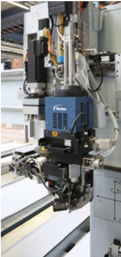
powerEdge with PU-melting unit: Edge banding with small glue joints and high moisture resistance
