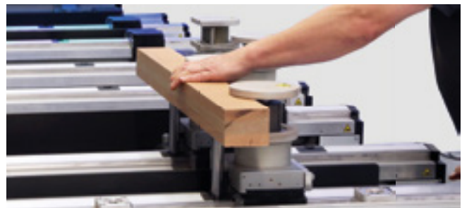
The stop bolts in the consoles guarantee accurate positioning of the clamping elements to ensure highly precise individual component production of window profiles without outside moulding and profiling of the frame. In addition, the stop bolts are used as an insertion aid for wide staves. This patented principle guarantees precise transverse profiling independently of the part width.
