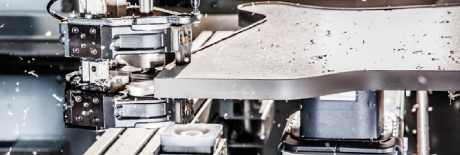
Scraping on inclined edges.
