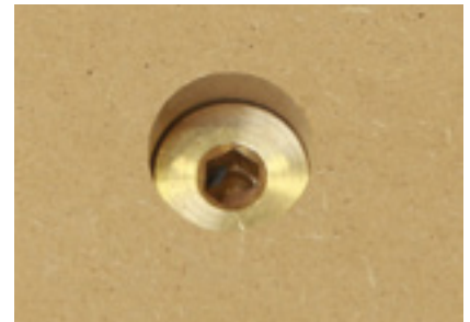
Hollow screws: Hollow screws for positive locking fixture of templates or dummy panels in the existing vacuum openings. In the version for template fixture, the vacuum can be routed via the borehole in the screw into the template.
