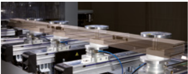
Sash bar insertion aid: Special inserts for sash bar clamping simultaneously act as insertion aids.
