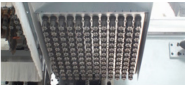
Drilling unit 144 spindles: Simultaneous drilling of 144 holes, for example when producing acoustic panels. Collet chucks for holding different shank diameters. Unit permanently mounted on the unit carrier.
