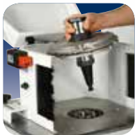
ISO 40 System rapid set up
