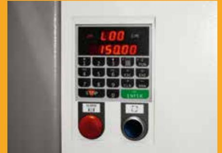
The thickener table electronic positioner, available on request, enables fast and precise worktable positioning. With calculator included.
