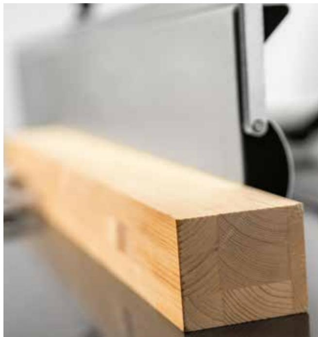
The fence with large surface enables to work with precision heavy and large workpieces.
