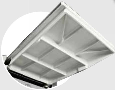
Strength and reliability: Surface tables are made with cast iron, ribbed for extra rigidity. Surface tables are precision ground and polished for a perfect finish and to facilitate stock feed. The long tables allow a perfect straightening also with very long workpieces.
