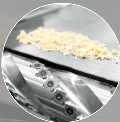
High finishing level: spiral spindle with knives.
