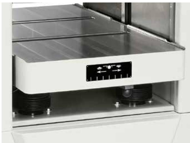
Working table with 2 idle rollers: machining of large sized pieces without problems thanks to the worktable with 2 idle rollers that facilitate feeding of large pieces. Available on request.
