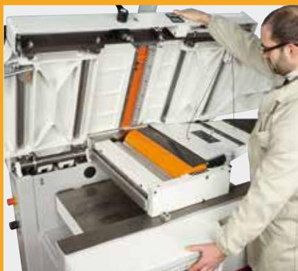
Change of processing in few seconds! Switching from surfacing to thicknessing, with the single surface tables opening action, we can automatically position the cutterhead protector and the dust hood.
