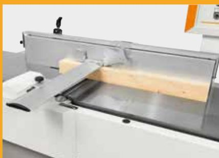
"TX MATIC" highest security: the "TX MATIC" cutterhead protection with automatic raise & fall adapts its movement during material feed. In this way the cutterhead is covered at all times, for enhanced safety.
