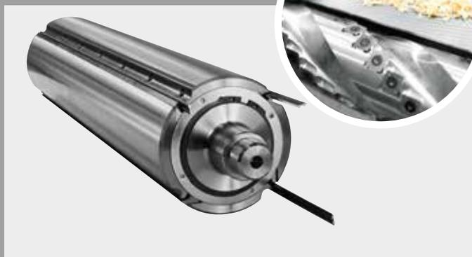
Both the PS 520 and PS 630 can be equipped with a Tera cutterhead and spiral spindle with knives.
