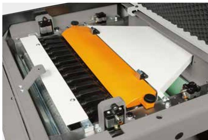
The PS 630 can be equipped, upon request, with pneumatic adjustment of the top feed rollers pressure from the front control panel rather than mechanical. The pneumatic pressure guarantees the same pressure with any stock removal.
