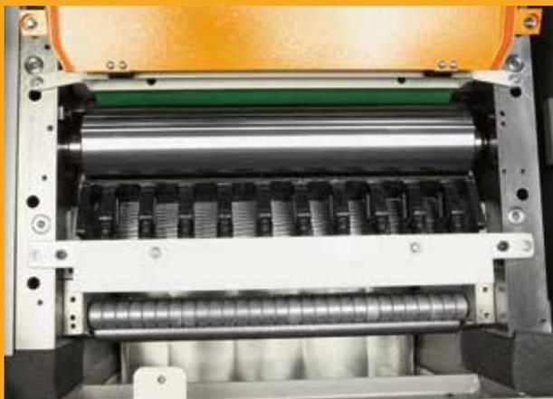
Planer unit with infeed anti kick-back fingers and segmented chipbreakers, serrated steel infeed roller with spiral teeth and rubber coated outfeed roller. Reduced noise level.
