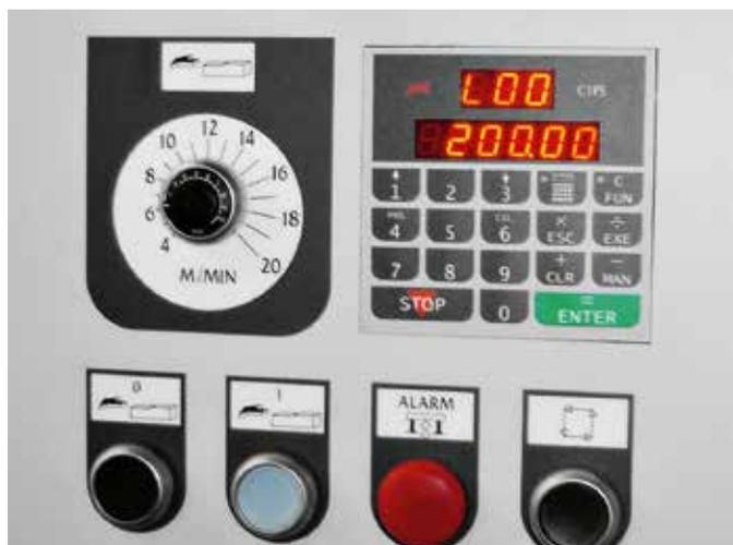
Fast and precise positioning thanks to one axis control that enables fast and precise worktable positioning. Control including calculator function. Available on request.
