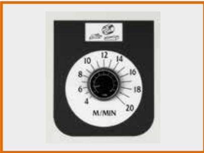
PS 630: Stepless feed speed adjustment through inverter from 4 to 20 m/min.
