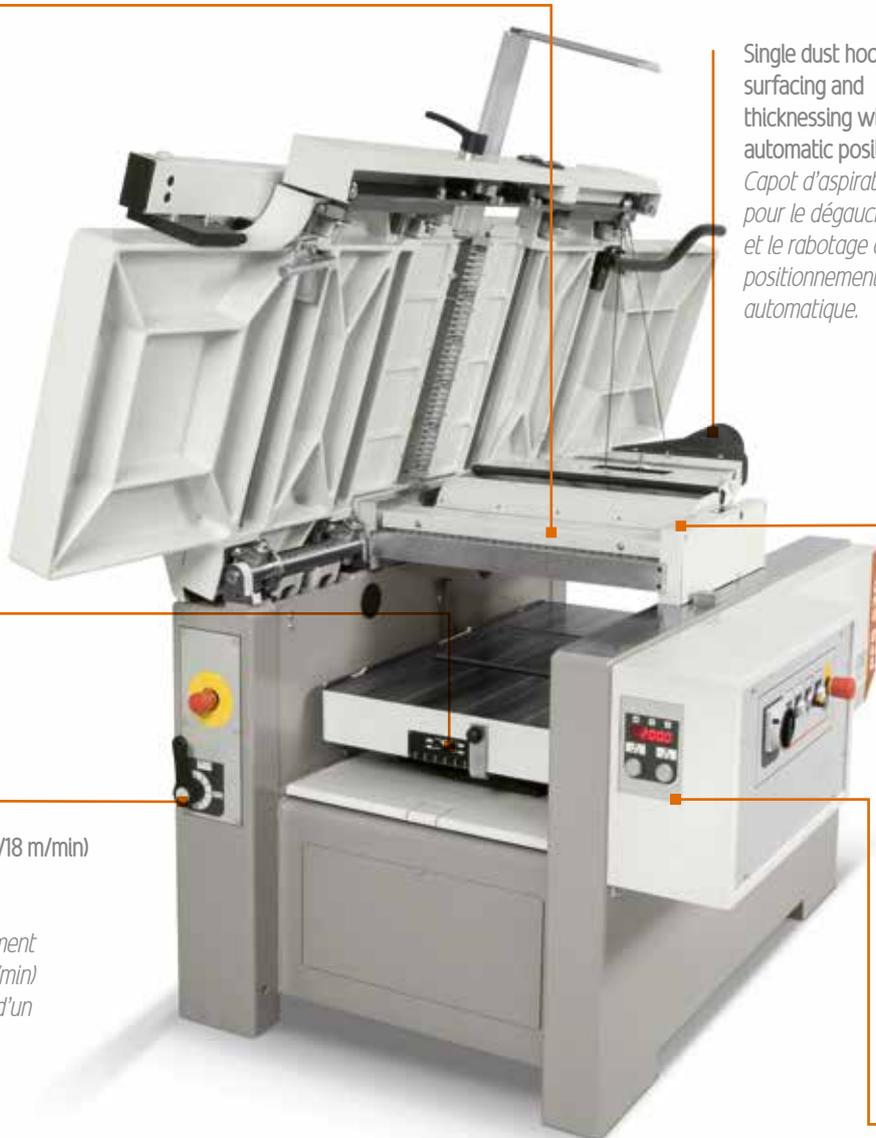
Powered thickening table raise & fall over 4 steel screws protected by dust.
