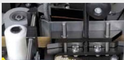
2 Edge feed for coiled and strip material
