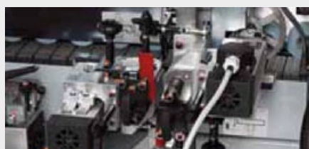
8 Multifunction trimming unit
