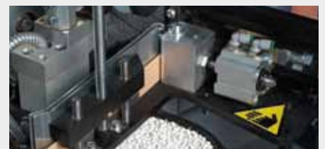
3 Edge feed for coiled and strip material
