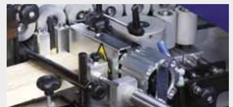
3 Edge feed for coiled and strip material (Image shown includes strip magazine)
