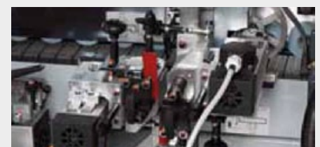
9 Multifunction trimming unit
