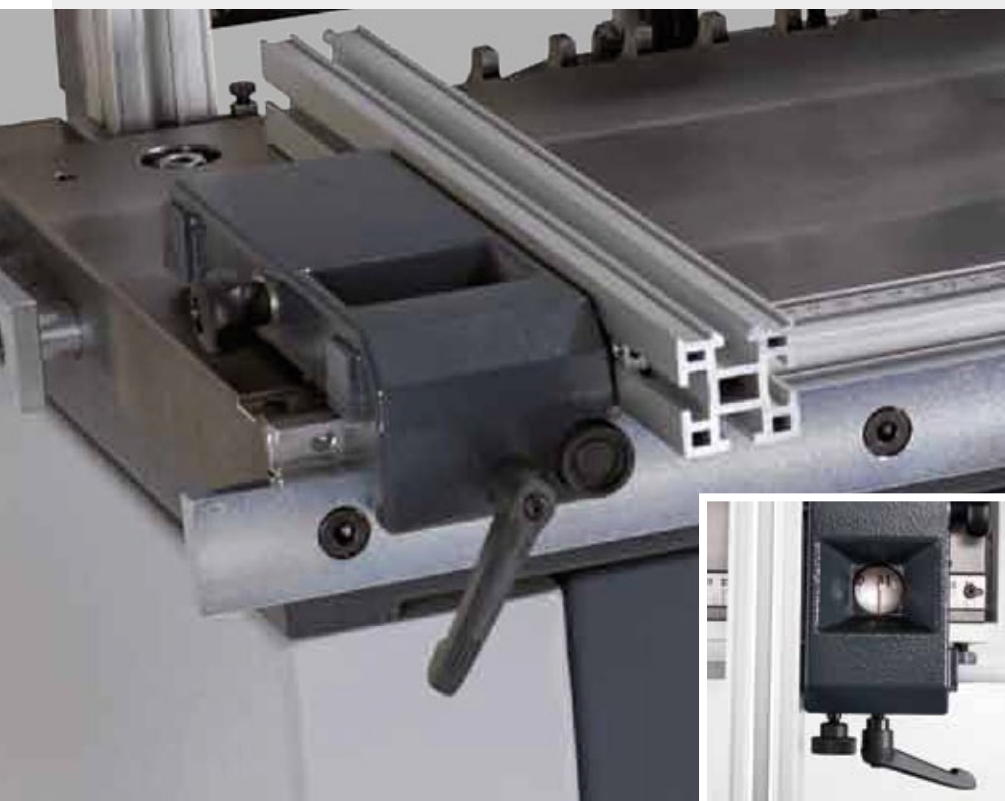
Solid side fences left and right with a profile of 420 mm.
