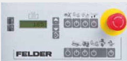
1 Operating panel with LCD display and keypad
