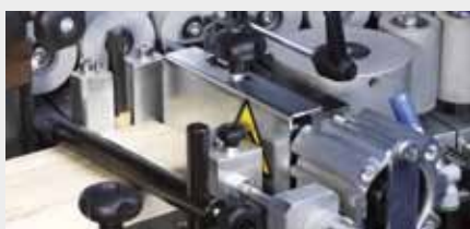
5 Guillotine scissors - Pneumatic pre-sizing (Image shown includes strip magazine)
