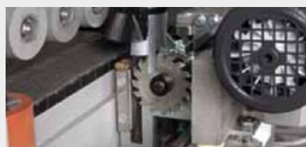
7 End trimming unit
