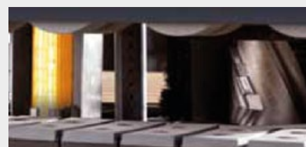
3 Infrared heating lamp (optional)
