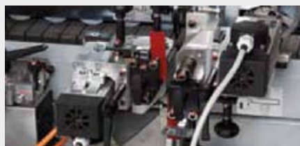
8 Multifunction milling aggregate
