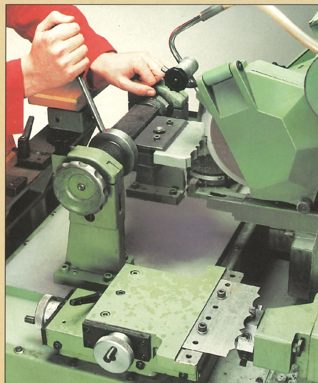
△ Jointer Stone Grinding. Profile jointer stones can be accurately cut to shape on a Wadkin Nx or Nxu profile grinder in a matter of minutes. The attachment also chamfers the stone ready for use.
