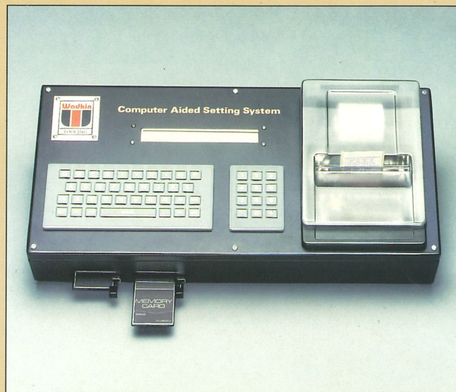
△ C.A.S.S. (Computer Aided Setting System) Information from the M.S.S. is automatically calculated and the CASS provides job details, cutterblock identification and actual horizontal and vertical dimensions. these can be transmitted to the moulder(s) in one or more ways:-
