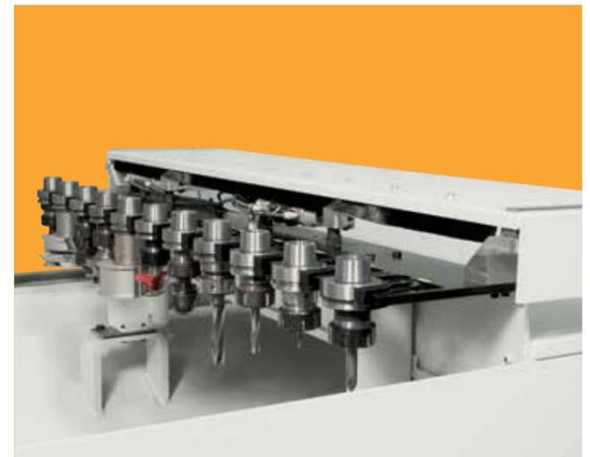
LINEAR T: tool changer on frame for large dimensioned tools with excludable covering for the maximum protection of the tools (Option).
