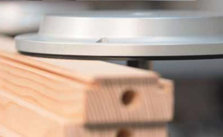
"Jet Fast" automatic positioning by NC. Quick positioning of the panel supports, suction cups and clamps. No intervention by the operator, max. precision and high flexibility.
