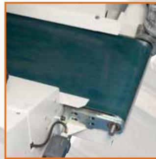
Off-cuts evacuation belt: optimal cleaning of the working area
